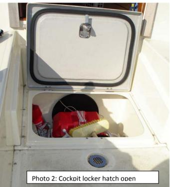
Let me just say this works really well and the locker is still huge; it runs the full length under the cockpit floor. As this photo shows, in addition to our battery and flares, all our warps and fenders, a bucket with our anchor warp in, you can also get a boat hook and brush in there
