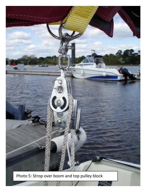
To this we attach a handy-billy. This is snap-shackled to the strop and we have a 360° swivel there which goes onto the top pulley block. This has two pulleys side by side and a jamming cleat. At the other end there is a single pulley with becket and a large snap shackle which goes onto the harness round the outboard.
