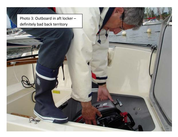
As we had a nice large flat cockpit area, we decided to simply lay the outboard on the floor of the cockpit. (Remember with this engine it has to be stored upright or flat. If flat the handle must be downwards). It can easily be hidden from prying eyes by a simple cockpit cover (wife currently working on posher Mark Two version) and secured by padlock to the strong point in the cockpit.
